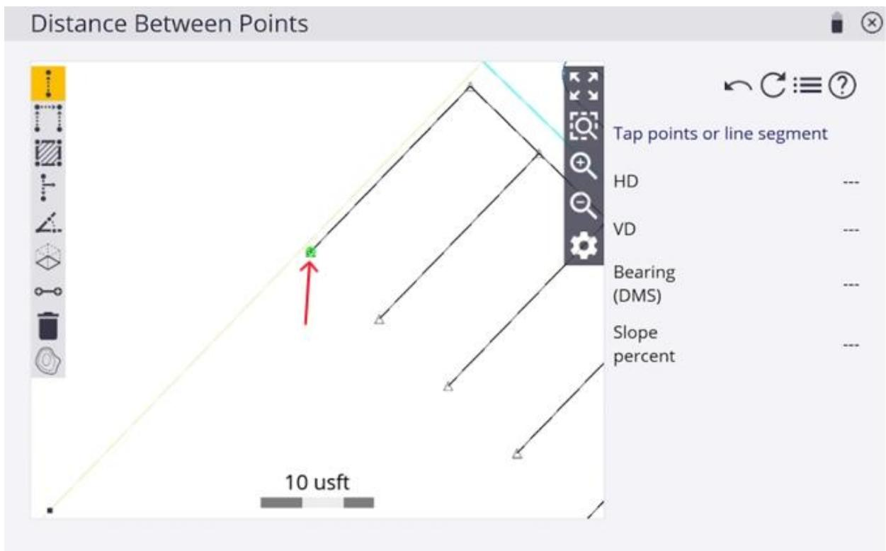
6. Select your second point, the HD is the horizontal distance, the VD is the vertical distance between the points. After verifying tap **ACCEPT**.
