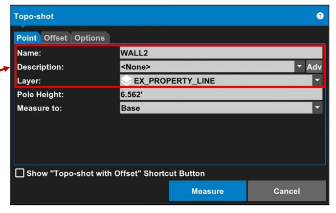
4. Leave the "Pole Height" to "6.562". (Check if your rod is snapped in place.) Then the "Measure to" is "Base".
