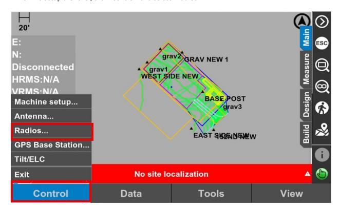
35. Set the Radio Type to the one used in the Rover, then click "Configure..."
