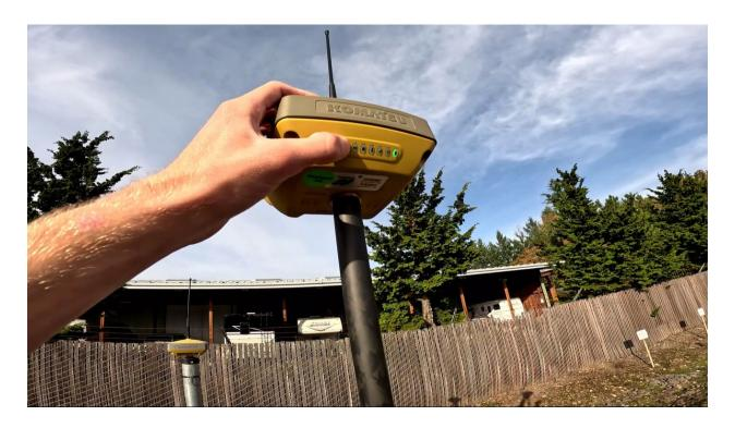
**3.** Make sure that your Base station is on a Base Post concreted to the ground. Turn it on by long pressing the power button.
