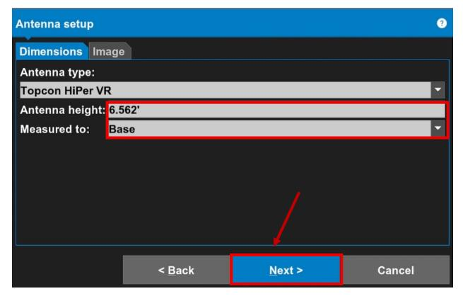
10. Setting the "Measured to" to "Base" means you will be measuring from the Base of the Rover to the Tip of the Rod as seen in the "Image" section.
