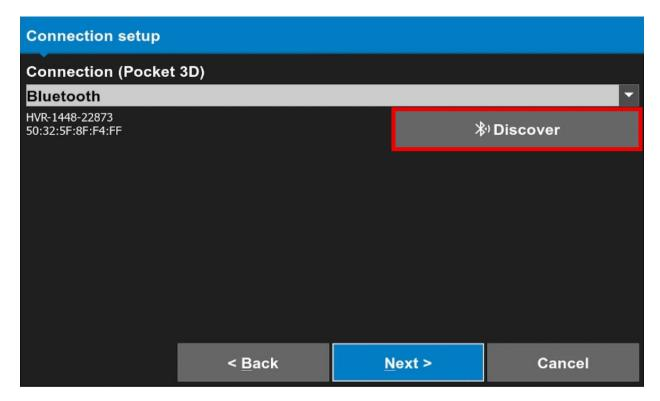
22. Click "Refresh" to find the Base and Rover. (Note: To identify your device, look underneath and find "SN" or Serial Number. Take note of the last four digits)
