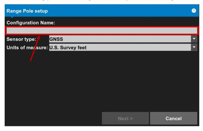
7. Set the Sensor type to "GNSS" and Units of measure to "U.S. Survey feet". Once done, click "Next"
