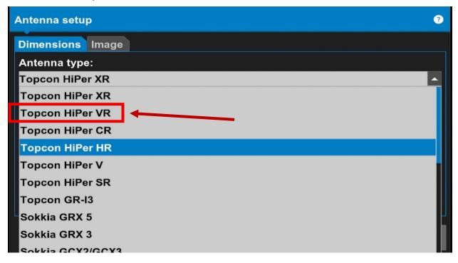
9. Keep the antenna height to **6.562'** and make sure it is Measured to **"Base"**. Click **"Next"**. **(Note:** If you have a different atenna height, you need to enter it manually)
