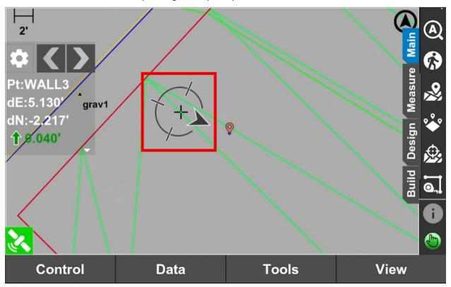
7. Make sure the equipment is in the center, and also make sure that the values are as close to zero. Once it's in the middle, mark your tip with a spray paint or any identifier available.
